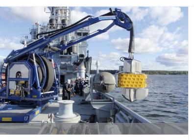
DSTI's rotary unions are suitable for the harshest offshore umbilical applications including installation, intervention, & workover.
