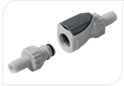
Figure 5: For applications requiring especially compact designs, today's non-spill couplings can connect tubing down to 1/16". Thumb latches ease operator use and provide audible confirmation that connection has been established.
