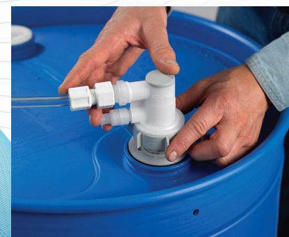
3. Turn the coupler locking ring clockwise until stop is reached (approximately 2 full turns); valve is opened during this process.
