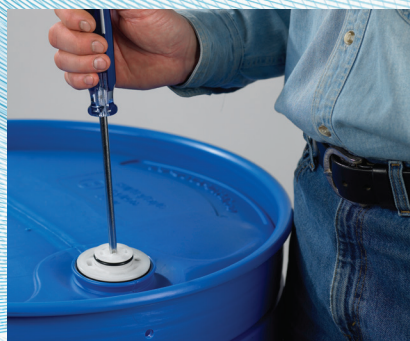
1. Turn shipping plug counterclockwise to remove. (Use a large flat blade, #4 Phillips screwdriver or coin.)
