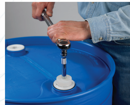
3. Torque insert with drum wrench or 1/2" drive torque wrench and a CPC torque socket tool (CPC PN 2408900).
