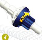
Twist the blue lock ring clockwise until the final audible "CPC Click" is heard (90° from the initial starting point). Alignment of the long blue lock ring rib indicator with the white body's rib indicator confirms initial rotation is complete.
