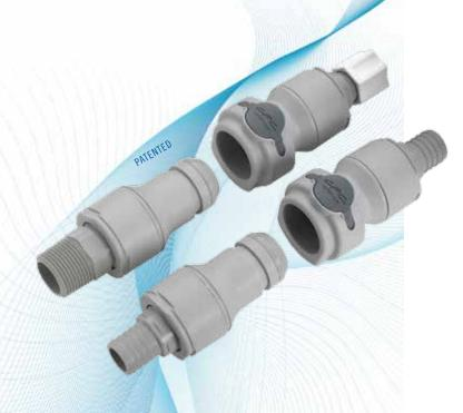
**NSH Series couplings** couplings are general purpose versions of our pressure-balanced, non-spill, ChemQuik® CQG06 couplings. Molded polypropylene, EPDM seals and a 100% springless and metal-free flow path provide broad chemical resistance and exceptionally high flow capacity, allowing instant disconnects (and reconnects), even under pressure. Their non-spill design virtually eliminates spills, minimizes downtime and enhances operator safety in a very low cost package.
