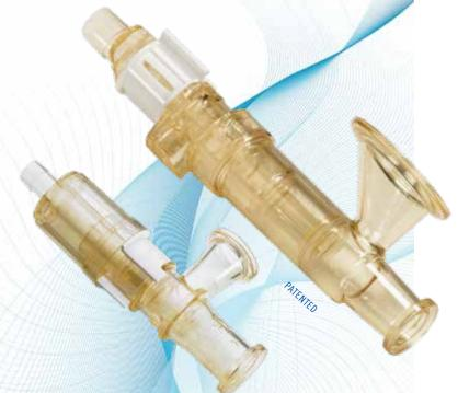
**Steam-Thru Connections** allow a quick and easy sterile connection between stainless steel biopharmaceutical processing equipment and disposable bag and tube assemblies. The single-use design saves time and money by eliminating unnecessary cleaning procedures and reducing validation burden associated with reusable components.
