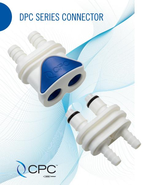
The 1/4" flow DPC Series couplings feature a dual port connection in a contoured design that delivers ease-of-use and excellent flow in a compact size. Made from acetal thermoplastic, the DPC Series includes valved and non-valved couplings with a single plastic thumb latch. One-hand operation makes the DPC Series the choice for simple, simultaneous connections and disconnections where two fluid lines are required.
