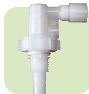
DrumQuik PUR Coupler Material: Virgin PVDF Spring: Virgin PEEK UHP (PPS or Teflon Encapsulated 316 SSt optional) Coupler Seals: FKM (Simriz FFKM optional)
