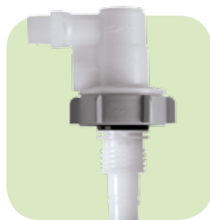
DrumQuik PRO Coupler Material: Virgin polypropylene Spring: 316 Stainless Steel (Hastelloy C optional) Coupler Seals: EPDM (FKM optional)
