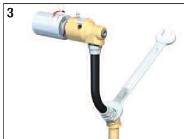
3 Connect flexible hose to supply line.
