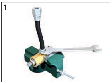
1 Mount housing in a bench vise and install hose.
