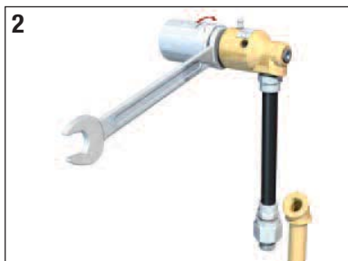
2 Install rotating union into machine.
